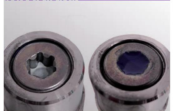
A screw in a verified component from a large batch (without and with TSS paint protection)
