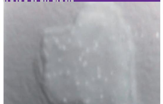
10x magnification of a photograph with colorless TSS paint protection applied
